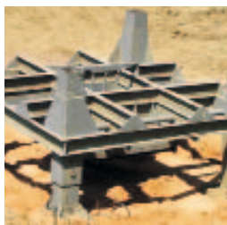
Bomb blast test (8 kg TNT) with Von Roll blast floor panel
